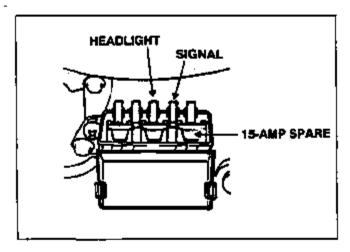
NOTE: The headlight fuse is being replaced with a 20-amp fuse because the spare fuse holder is limited to three fuses. This will give the owner access to a replacement fuse of the proper type for either the brake/taillight or headlight circuit. The higher amp fuse does not compromise the headlight circuit in any way.
